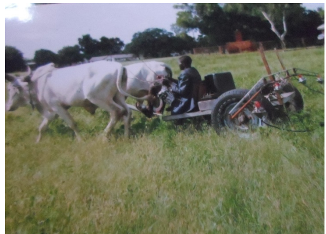
Plate 3: Animal Drawn Ground Metered Shrouded Disc Sprayer in Operation
