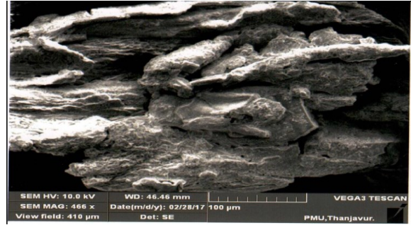
Fig. 4B. SEM images of Iron oxide nanoparticles synthesized using Leucas aspera leaf extracts at 410μm magnification levels
