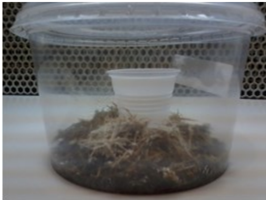
Fig. 1. Experimental unit for microbial respiration mediation containing a small wide mouth container containing 10mL of NaOH (2N).
