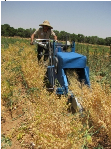
Fig.6. Harvest operation by prototype chickpea harvester
